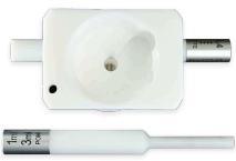
Measuring cell 1 ml and 3 ml with pestle
