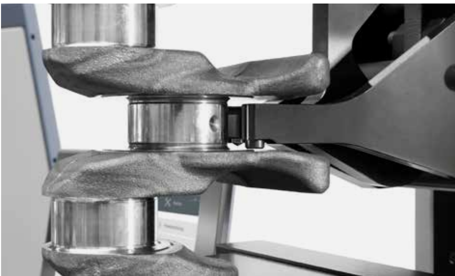
INDENTOR EXTENSION FOR HARD-TO-REACH TEST LOCATIONS
